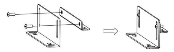
**Note:** You can adjust the bracket anywhere along the axis of the hole connecting the pieces allowing a flush fit with the wall or enclosure the unit is installed on.
